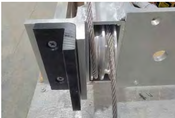
Lift corners are made from UHMW plastic for smooth operation
